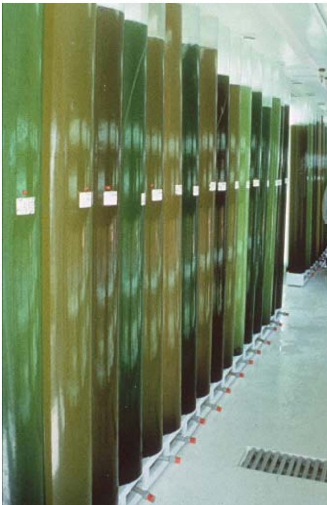
Figure 2.7.b. Batch culture systems for the mass production of micro-algae in 150 l cylinders.
