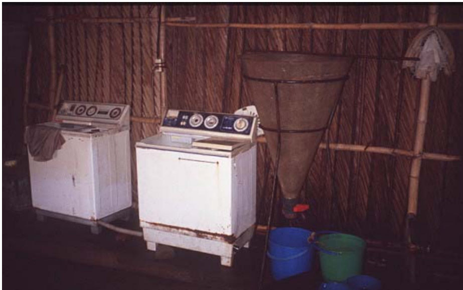
Figure 4.5.27. A vertical spin dryer (for removal of excess water) and a transparent conical shaped tank with a bottom valve (for density separation).
