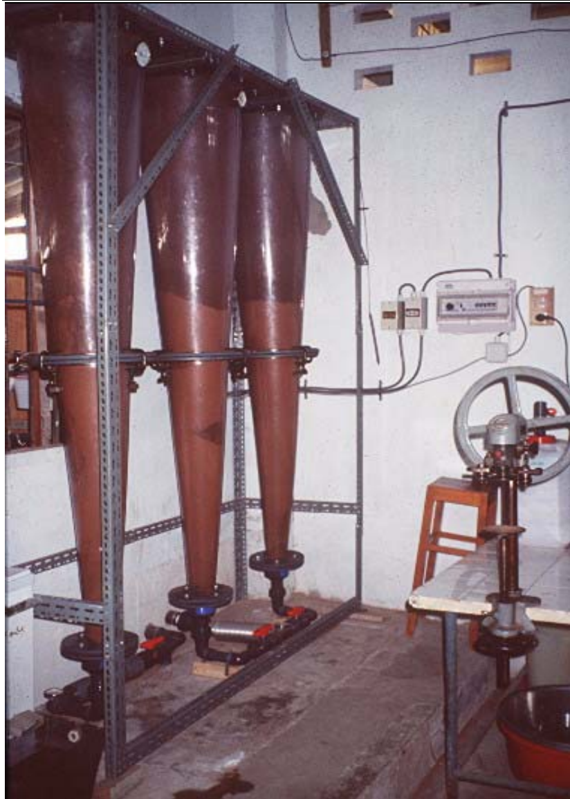
Figure 4.5.20. A fluidized bed dryer for Artemia cysts.
