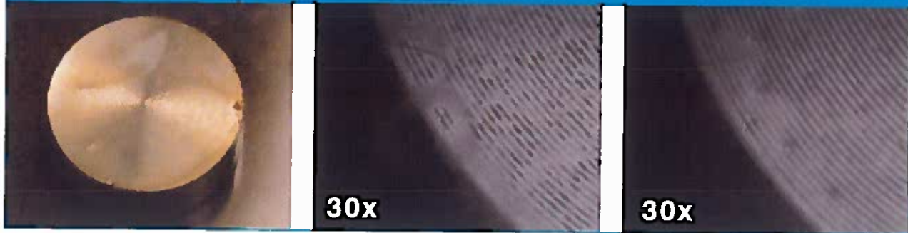
Fig. 3 a-c: Photograph of a) CDC biofilm reactor disc; b) P. aeruginosa cultured on the CDC Biofilm Reactor disc; c) P. aeruginosa CDC Biofilm Reactor Disc after cleaning with a formulated alkaline cleaner
