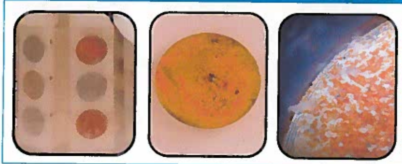
Fig. 4a-c Photograph of a) Both rouged and passivated CDC biofilm reactor discs in CDC biofilm reactor, b) P. aeruginosa cultured on rouged CDC biofilm reactor disc, c) P. aeruginosa cultured on rouged CDC biofilm reactor disc under 30x magnification
